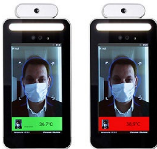
Fig. 1: Infection prevention in companies and the public sector: The ICS body temperature screening system measures the human body temperature automatically, contactless, and within two tenths of a second.
